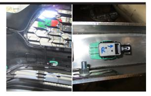
CAUTION: Care must be used to not glue the sensor to the mounting bracket. This will cause sensor failure.
